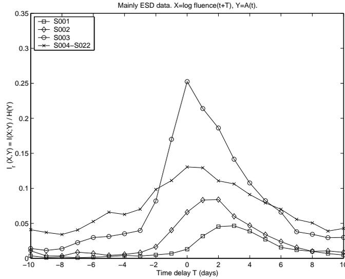
Figure 2.4: The relative mutual information  $I(X; Y)/H(Y)$  for the different anomaly sets as a function of log daily  $> 2$  MeV electron fluence delayed -10 to 10 days. A subset of the anomaly data is selected that mainly related to ESD as explained in the text.
