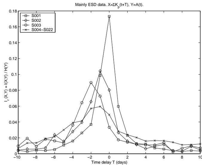
Figure 2.3: The relative mutual information  $I(X;Y)/H(Y)$  for the different anomaly sets as a function of  $\sum K_p$  delayed -10 to 10 days. A subset of the anomaly data is selected that mainly related to ESD as explained in the text.
