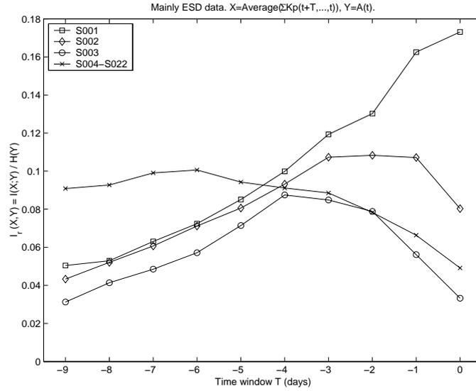
Figure 2.2: The relative mutual information  $I(X;Y)/H(Y)$  for the different anomaly sets as a function of the average  $\sum K_p$ , where the average goes from 1 to 10 days. A subset of the anomaly data is selected that mainly related to ESD as explained in the text.
