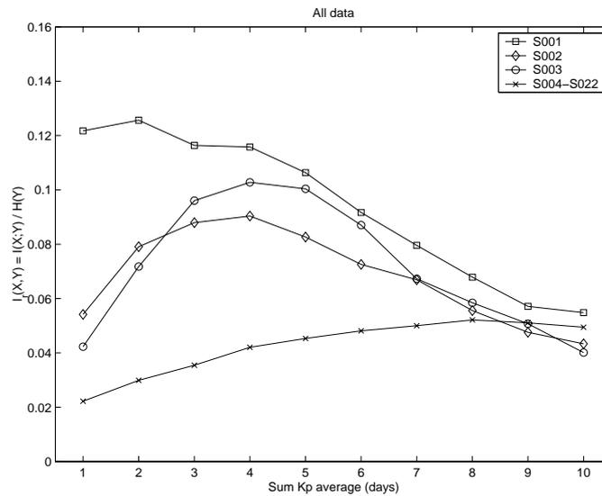
Figure 2.1: The relative mutual information  $I(X; Y)/H(Y)$  for the different anomaly sets as a function of the average  $\sum K_p$ , where the average goes from 1 to 10 days. The anomaly sets contain all the anomaly data.
